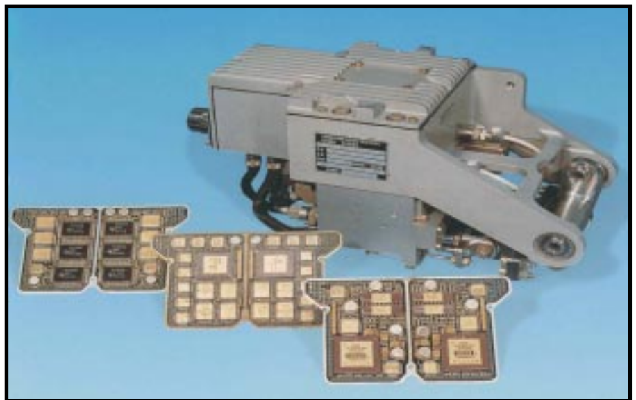
Photo 2—In especially harsh environments, the control electronics may become a part of the hydraulic actuator. The advantage is that there needs to be very few electrical connections with the outside world. Besides power, everything else can be fiber optics. This actuator won't stop working even during nuclear explosions, which are notorious for their high-power EMP.
