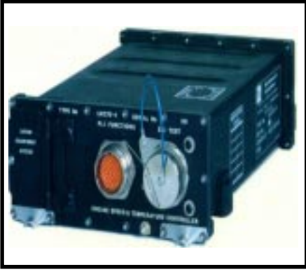
Photo 1— To protect an electronic controller from the effects of harsh environment, its package looks like a brick, yet it is deceptively light because it is usually machined out of a solid piece of aluminum. You can drive over this baby with a truck or dunk it in the water and it won't lose a beat.
