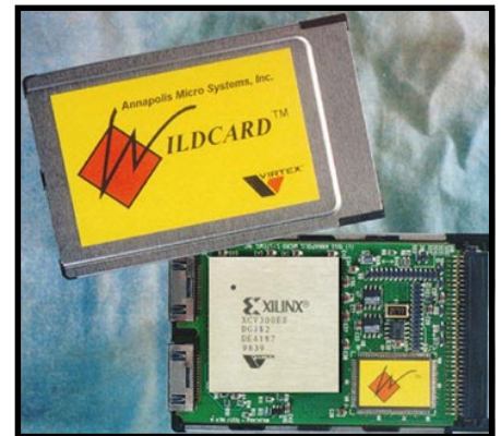
Photo 1—The Wildcard from Annapolis Micro Systems puts a big chip (Xilinx XCV300) in a small package.
