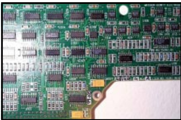
Photo 1 —Here you can see a partial view of an autorigging module implemented with traditional SSI and MSI logic circuits. Components are mounted on both sides of this SMT circuit board. How would you like to troubleshoot this circuit?
